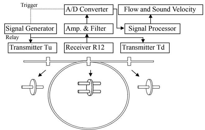
Fig.5. Schematic diagram of a newly designed ultrasonic flowmeter
