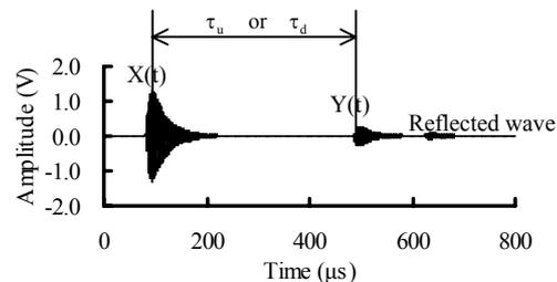
Fig.6. Ultrasonic signals of designed ultrasonic flowmeter
