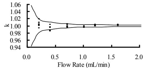
Fig.9. Calibration results at 25 MHz sampling frequency
