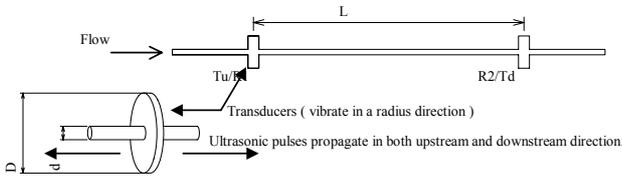
Fig.2. Attachment of a transducer to a measuring pipe
