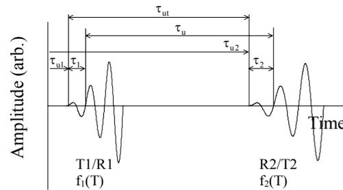
Fig.3. Ultrasonic signals propagated from Tu to R2 along the flow direction
