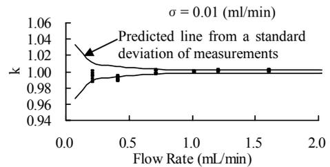
Fig.8. Calibration results at 100 MHz sampling frequency
