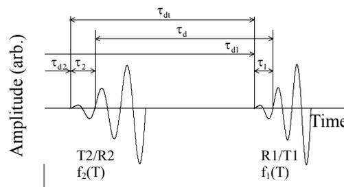
Fig.4. Ultrasonic signals propagated from Td to R1 against the flow direction
