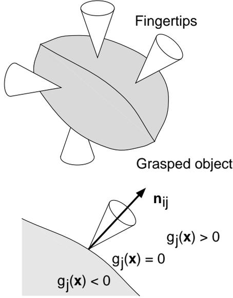
Fig. 1 Model of grasping by robotic hand
