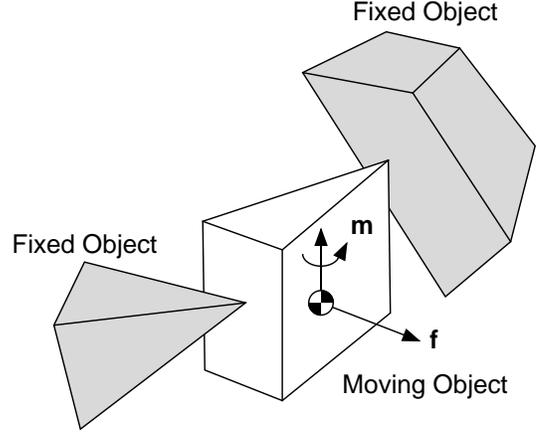
**Fig. 3** Moving object constrained by contact with fixed objects
