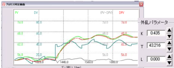
Fig 8(d) D(s) Identification Result for first order lag and dead time process
