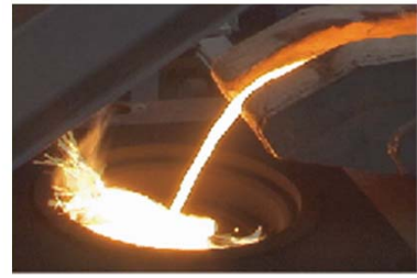
Fig. 9 Splash on Pouring in Press Casting Process
