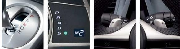
Fig. 4 Manual gear-shift interfaces
