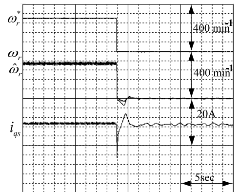
Fig. 12 Step response with \varepsilon_1 -modification approach (2) (with observer gain, 50% load)
