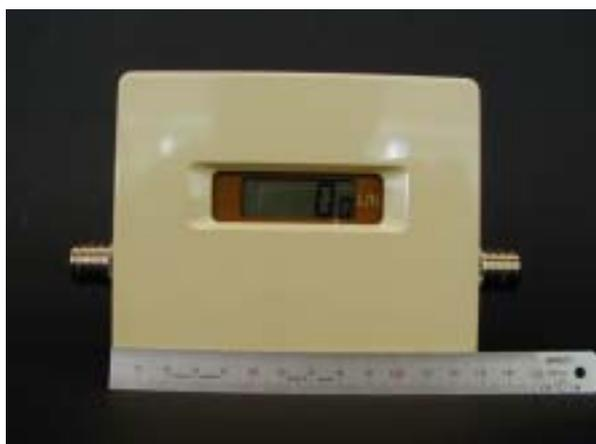
Photo3 The photograph of the instantaneous flow meter using the MEMS flow sensor.
