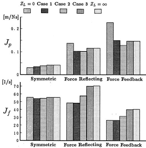
Fig. 3 Numerical example of maneuverability index
