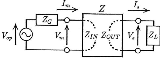
**Fig. 2** Connection of power source and load to two-terminal-pair network.
