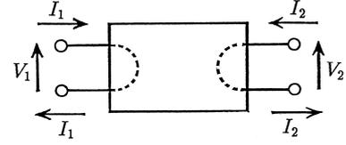
Fig. 1 Two-terminal-pair network.
