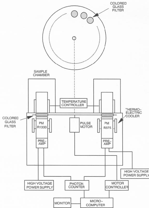
**Fig. 1** Block diagram of the filter-differential type biophoton spectral analyzer system.
