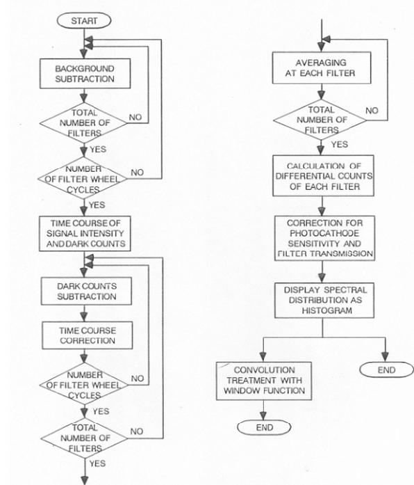
**Fig. 2** Flow chart for extracting the spectral information in the filter-differential type biophoton spectral analyzer system.
