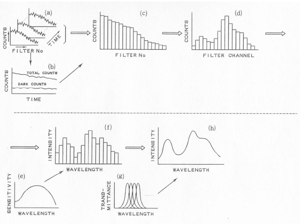
**Fig. 3** Schematic illustrations of the data processing in the filter-differential type biophoton spectral analyzer system.
