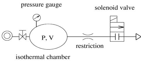
**Fig. 2** Experimental apparatus for the temperature measurement (the case of discharge)
