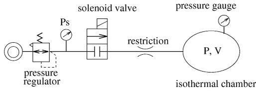
**Fig. 1** Experimental apparatus for the temperature measurement (the case of charge)
