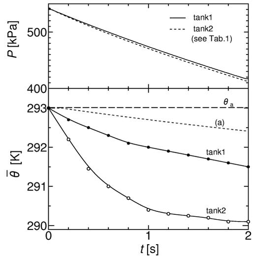
(a)temperature response assuming that the whole heat generated by the expansion of air was transferred to the material
