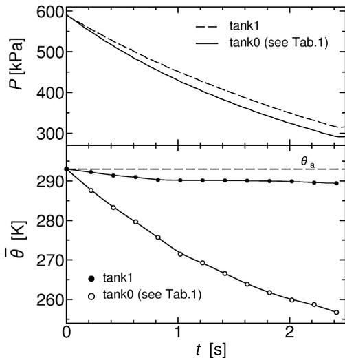
**Fig. 3** Temperature changes during discharge
