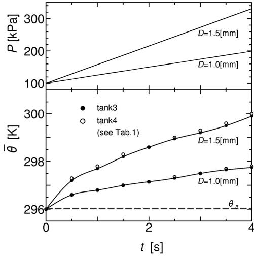
**Fig. 5** Relation between the shape of the chamber and the temperature change
