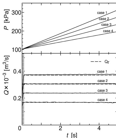
Fig. 9 Experimental results of the steady flow rate measurement
