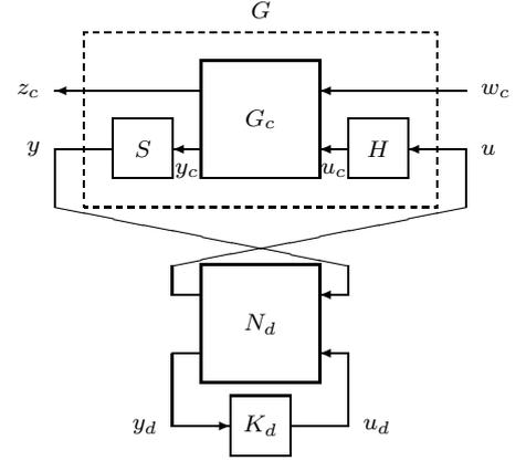
Fig. 2 Sampled-data system with periodic discrete-time components
