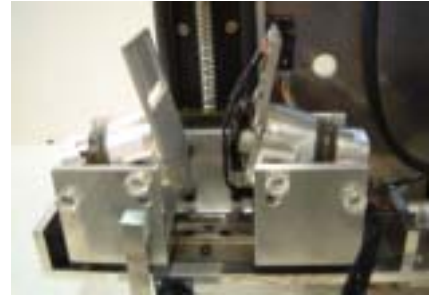
(b) Close-up ultrasonic vibrator and force sensor
