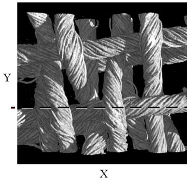
**Fig. 11** Structure of double-layered woven fabric reconstructed by directly accumulating the CT images (dotted line indicates the portion for which the CT image of Fig. 10 is used)
