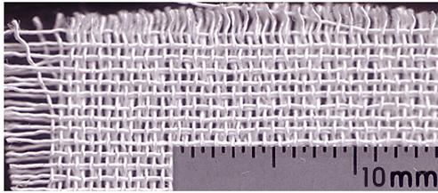
**Photo. 2** Photograph of the double-layered woven fabric sample
