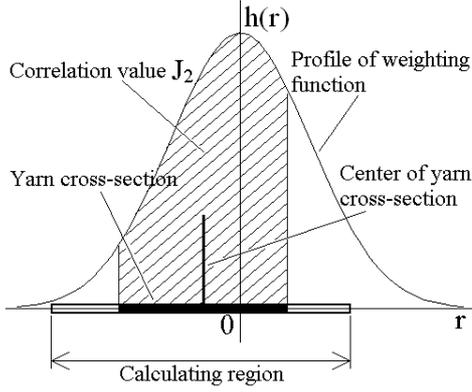
**Fig. 2** Profile of the weighting function  $h(r)$ , the yarn cross-section, its center, the calculating region, and the correlation value  $J_2$ , which are described in two dimensions, respectively
