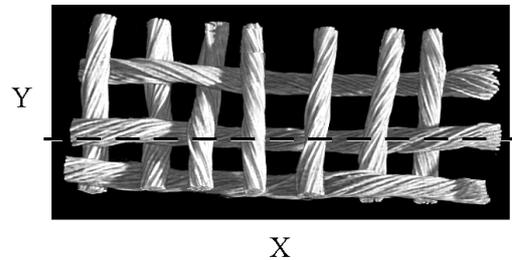
**Fig. 4** Twill structure reconstructed by directly accumulating CT images (dotted line indicates the portion for which the CT image of Fig. 3 is used)
