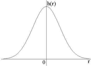
**Fig. 7** Profile of the weighting function of the yarn cross-sectional model,  $h(r) = \exp\{-s r^2\}$
