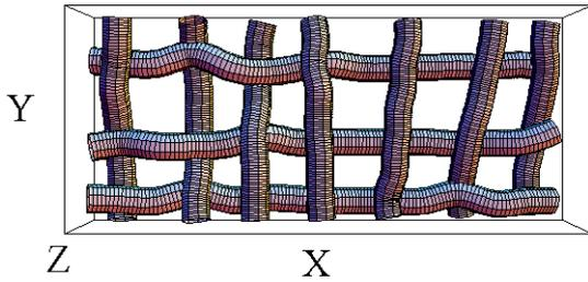
**Fig. 5** Twill structure reconstructed from the positional information of each yarn estimated by the yarn cross-sectional model correlation method
