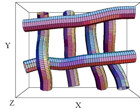
**Fig. 13** Independent expression of the warp of the under layer and the weft of the upper layer of a double-layer woven fabric sample
