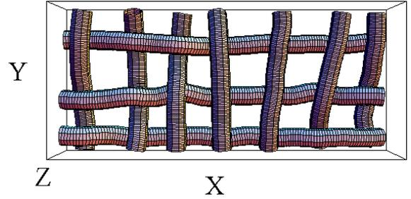
**Fig. 9** Twill structure reconstructed from the positional information of each yarn estimated by the yarn cross-sectional model correlation method using the improved weighting function
