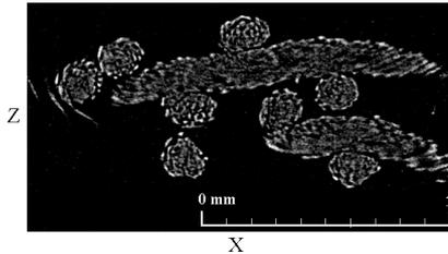
**Fig. 10** Example CT images of the double-layered woven fabric sample
