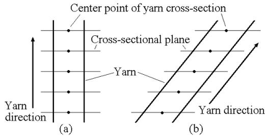
**Fig. 1** Schematic diagram of the relationships between a cross-sectional plane and a yarn direction, where (a) the cross-sectional plane is perpendicular to the yarn direction and (b) the cross-sectional plane is slanten-dicular to the yarn direction
