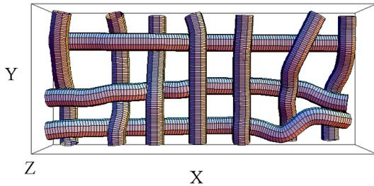
**Fig. 6** Twill structure reconstructed from the positional information of each yarn estimated by the cross-sectional images correlation method
