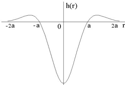
**Fig. 8** Profile of the improved weighting function of the yarn cross-sectional model,  $h(r) = -2 \exp\{-s r^2\} + \exp\{-t r^2\}$
