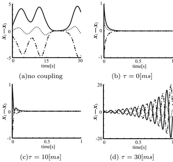
**Fig. 5** Time responses of the state differences  $x_1 - x_3$  with  $x_{11} - x_{31}$  (—),  $x_{12} - x_{32}$  (·),  $x_{13} - x_{33}$  (---).
