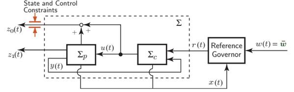
**Fig. 2** Closed-loop systems equipped with reference governor
