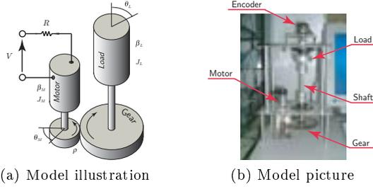
Fig. 4 Position servomechanism
