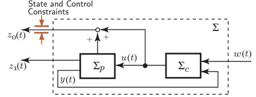
Fig. 1 Closed-loop systems with state and control constraints
