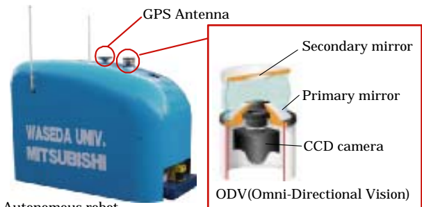
Fig.2 Robot with high-accuracy positioning and omnidirectional vision.
