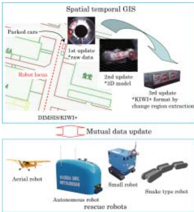
Fig.1 Spatial temporal GIS update method using rescue robots.
