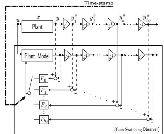
Fig. 4 Augmented system and gain switching observer
