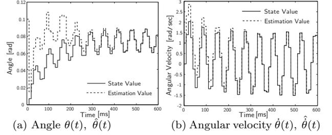
**Fig. 8** Time response of state and estimation value ( $r = 1.0$ )
