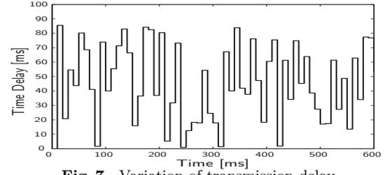
**Fig. 7** Variation of transmission delay
