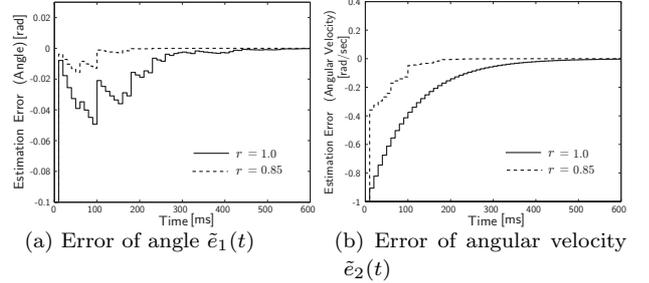
**Fig. 10** Comparison of estimation errors ( $r = 1.0, 0.85$ )
