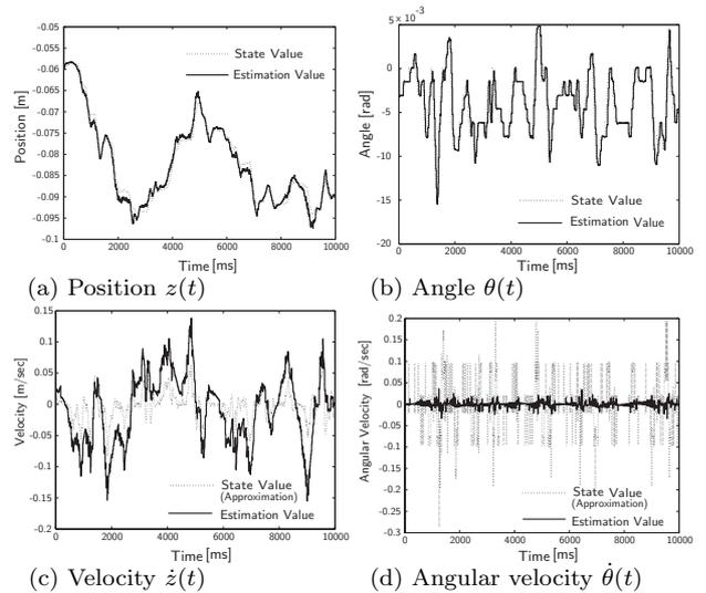
**Fig. 12** State estimation of an inverted pendulum
