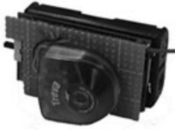
Fig. 7 Prototype sensor node with embedded camera
