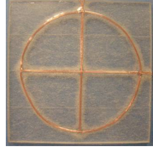
Fig. 3 The sensor unit consisting of a loop coil for measuring H_z and two gradiometers for measuring \frac{\partial H_z}{\partial x} and \frac{\partial H_z}{\partial y}
