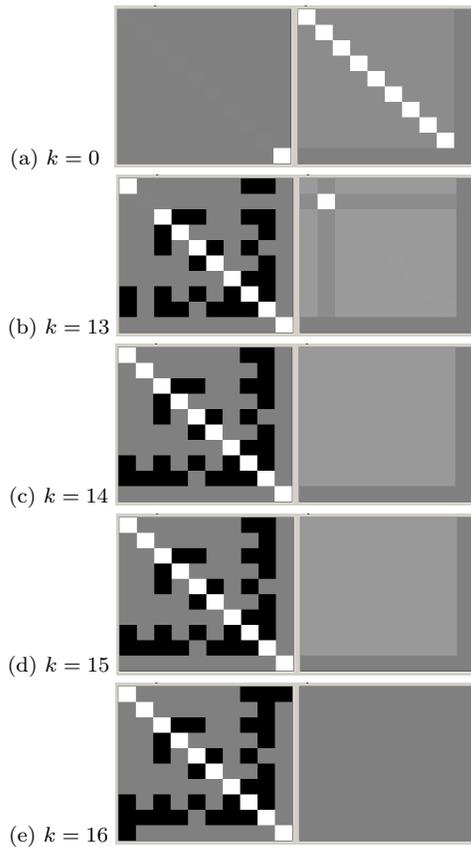
**Fig. 5** Brightness view of  $\Sigma_k^{-1}$  (left) and  $\Sigma_k$  (right) for the experiment in Fig.4. At  $k = 14$ , all the sensors except one finished coupling and the corresponding elements of  $\Sigma_k$  became flat although the values were nonzero. At  $k = 16$ , one of the sensors encountered the sensor 10 with an accurate clock. Then all the elements of  $\Sigma_k$  vanished, which means all the sensors were adjusted at a time to the sensor 10.
