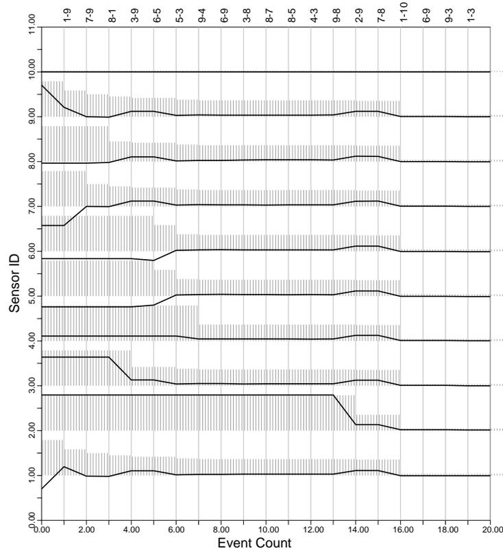
**Fig. 4** An example of result. Except for sensor 10, offset times are assumed to be biased, hence  $\Sigma_k$  is still large after the synchronization from 1 to 9 has completed. At  $k = 16$ , one sensor encountered the sensor 10 with an accurate clock, then all the offset times including the bias became zero at a time.
