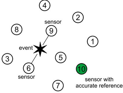
**Fig. 1** Situation of the problem. Most sensors in a network are uncalibrated/unsynchronized although some may be accurate. The inconsistency is detected only when two sensors of them detect eventually the same event.
