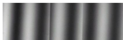
Fig. 2 Interferogram with carrier fringes.
