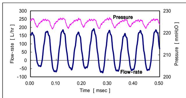
Fig.3 The flow and pressure waveforms measured pulsating flow using the instantaneous gas flow meter.
