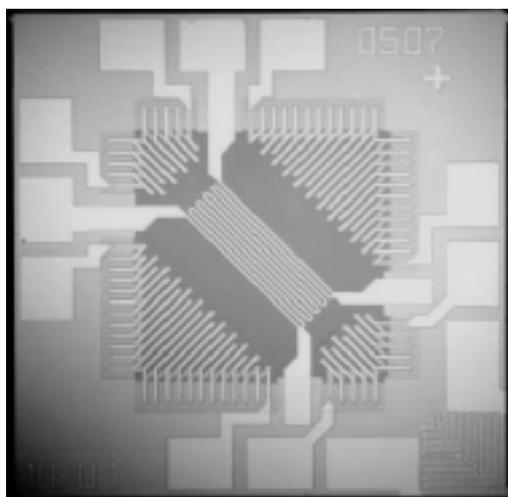
Photo2 The photograph of the MEMS flow sensor using four thermopiles as a flow rate monitor and a temperature distribution monitor.
