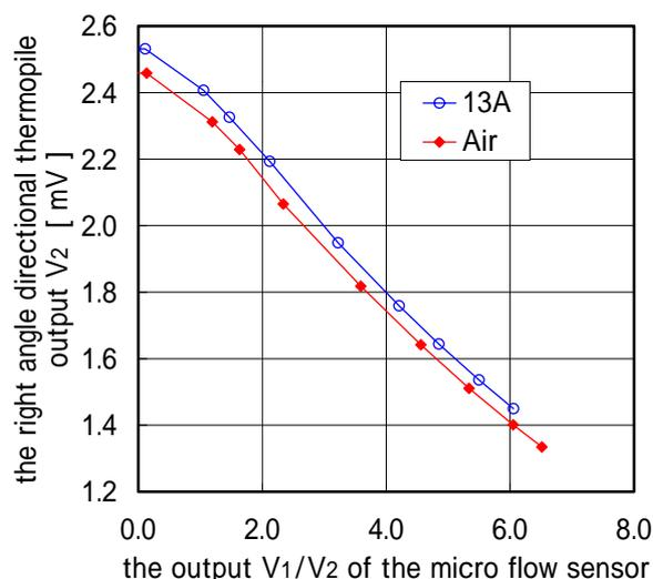
Fig.8 The relationship of the right angle directional thermopile output against the flow rate sensing.
