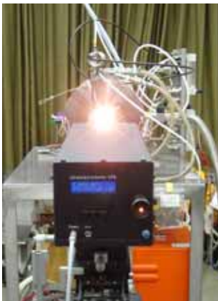
High temperature fixed-point blackbody furnace using metal-carbon eutectics. (Courtesy: NMIJ, AIST)
