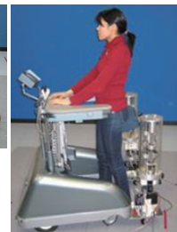
(Left) New mobility-aid vehicle controlled by walking (Middle) Walking assistive robot with a weight-holder under the Ischia
